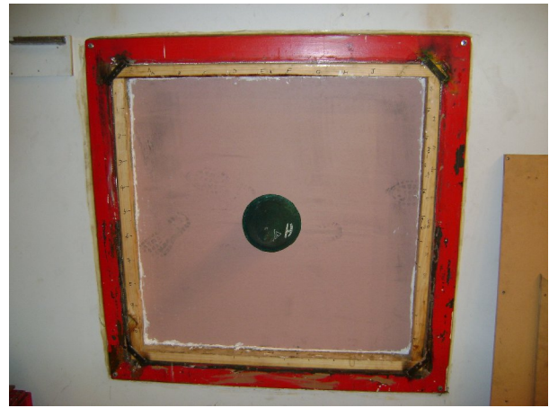
Figure 2.3: Downlight Mitt (covering downlight) installation on plasterboard (from source chamber)
