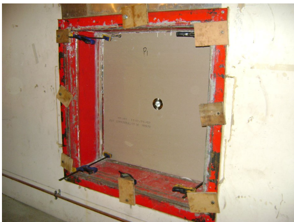
Figure 2.2: Downlight installation in plasterboard (from receiving chamber)
