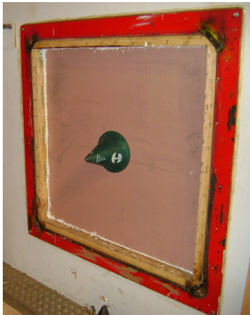
Figure 2.3: Downlight Mitt (covering downlight) installation on plasterboard (from source chamber)
